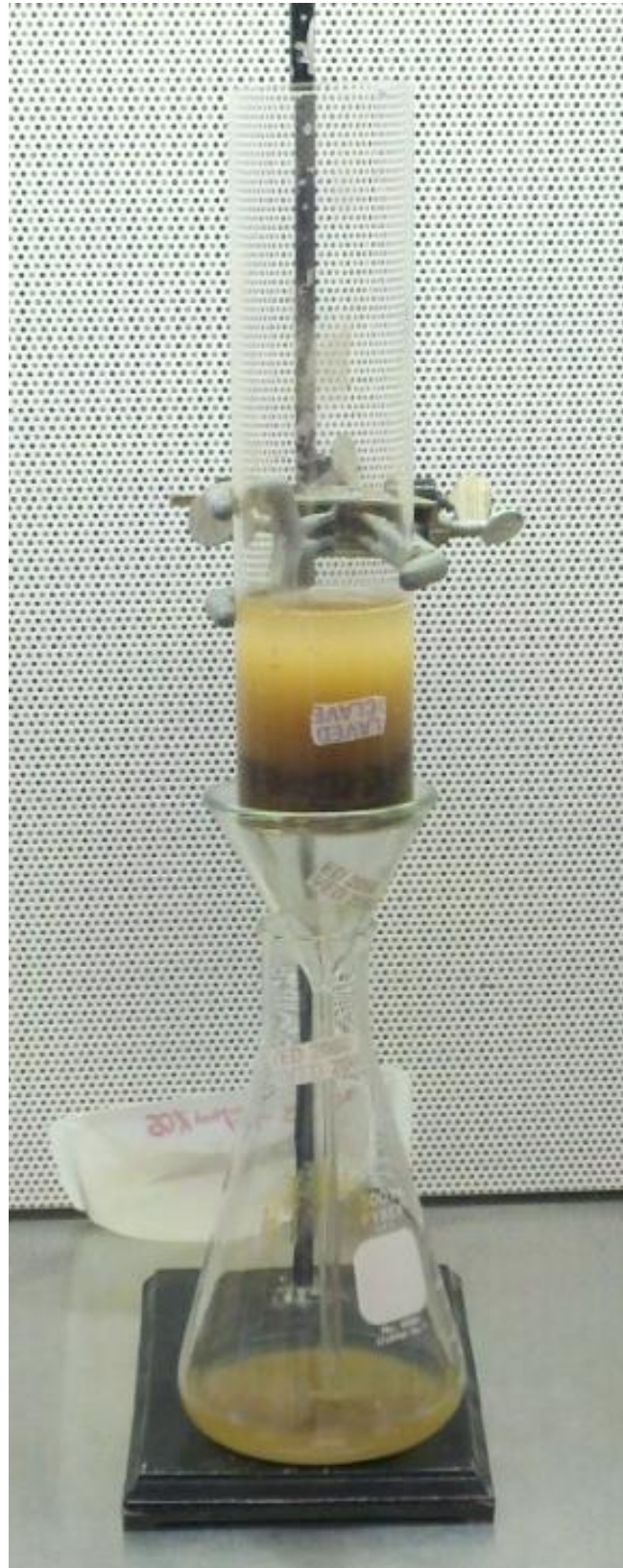
Figure 2. A photograph of the set up for flowing and collecting fluid for bacteria data
